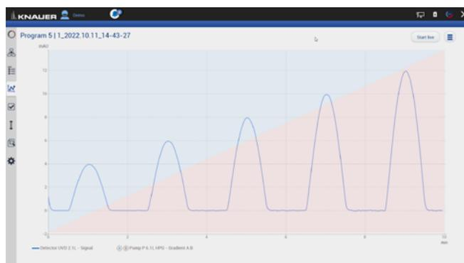
**Fig. 8-10** Chromatogram shows UV signal and gradient composition
