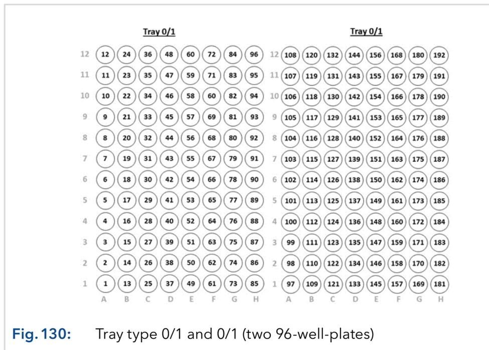
**Fig. 130:** Tray type 0/1 and 0/1 (two 96-well-plates)
