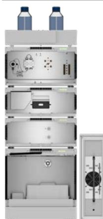
**Fig. 20** System setup; from top to bottom: eluent tray with bottles, pump, diode array detector (DAD), refractive index detector (RID), autosampler, right: oven.
