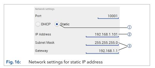
**Result** The device is now accessible via the static IP address.
