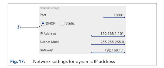
**Result** The device is now accessible via a dynamic IP address.
