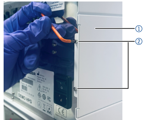
Fig. 1: Removing the two screws on the back of the device
